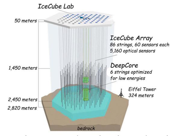
IceCube detects these neutrinos by detecting the light released when they interact with the ice. This light is called Cherenkov radiation.
